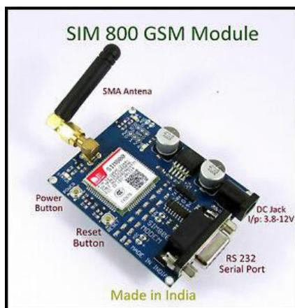
Fig 7. GSM SIM 8000A
