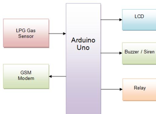
Fig 1.Process Diagram
