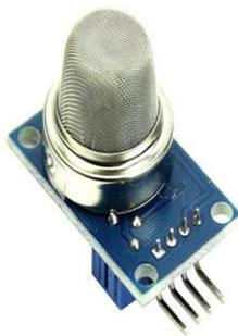
Fig 3. Gas Sensor (MQ 6)
