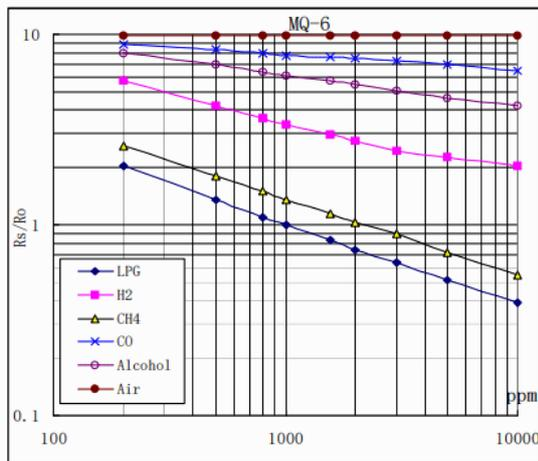
Fig 4.shows the typical sensitivity characteristics of the MQ-6 gas sensor for several gases.
